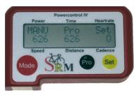
For a manual comparison turn the unloaded crank in a clockwise direction to switch the PowerMeter on.
