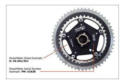
You can find the correct PowerMeter slope located-at:
