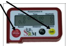
Push, simultaneously, **MODE** and **SET** to switch the PowerMeter's display to calibration mode
